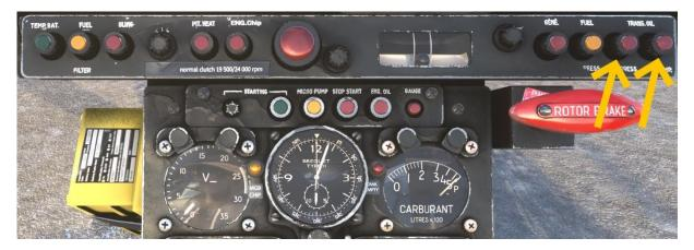
This will result in a complete loss of power on the main rotor and you have to initiate an autorotation landing.
