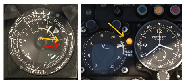
As a consequence, metal chips in the transmission oil will be detected and the **MGB CHIP DETECTOR** warning light on the main instrument panel illuminates.
